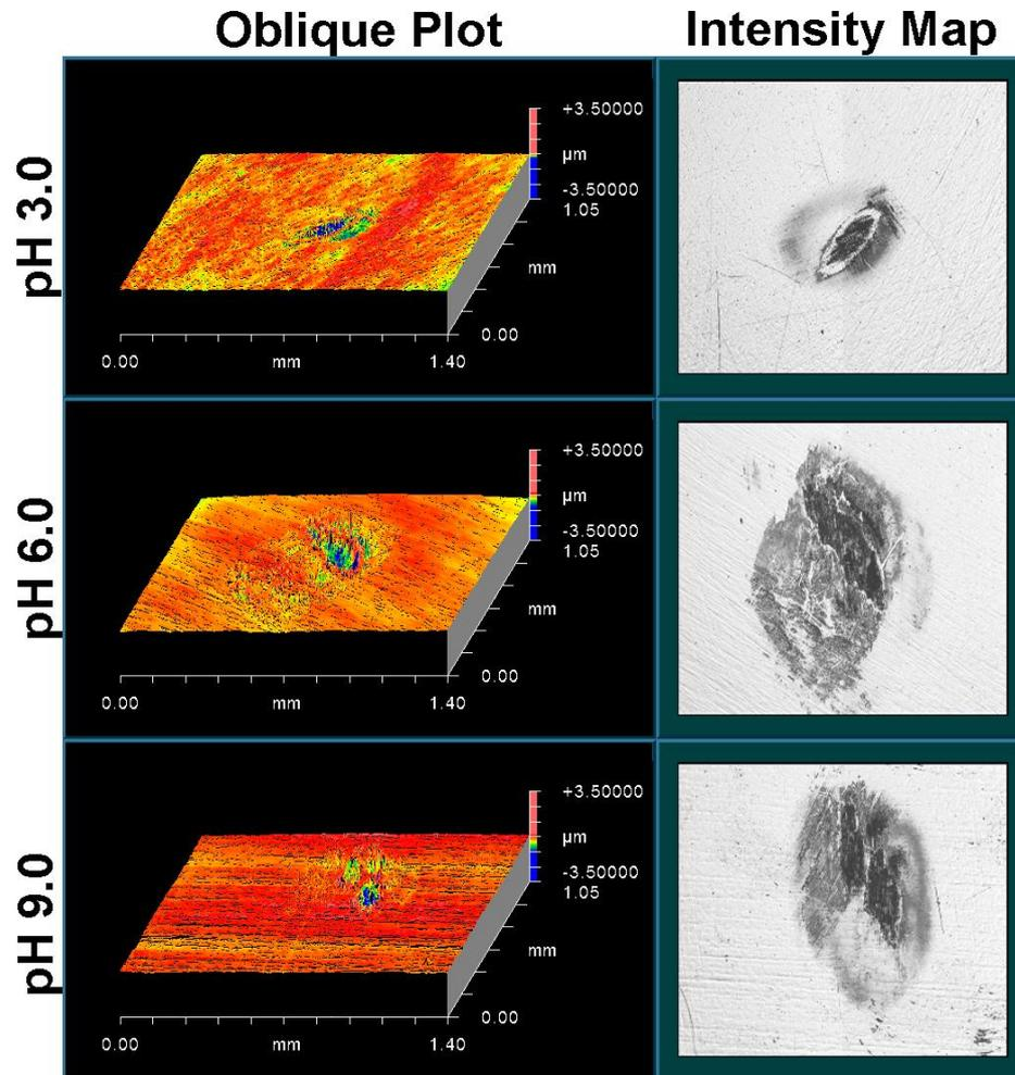
**Fig. 1 – Zygo images of wear scars on Ti6Al4V alloy formed with a 5N load with a 1 Hz frequency.**
